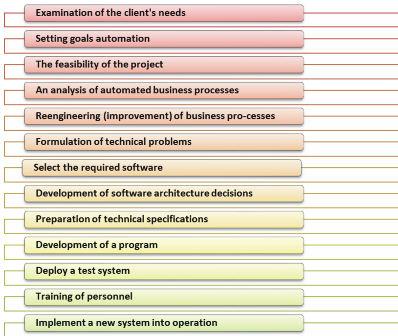
Fig. 3. Smart automation steps (adapted according Ref. [10].)
